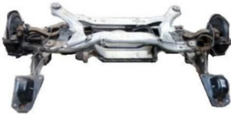
**Susp. trasera completa desmontada (aluminio)**
